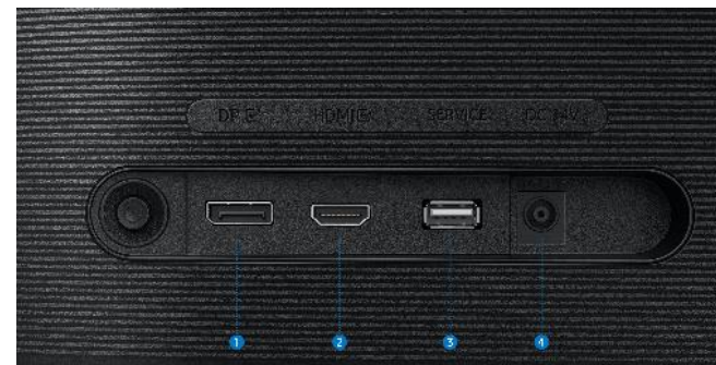
1 DisplayPort IN 2 HDMI IN 3 USB/SERVICE 4 DC14V
